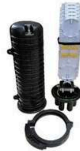
Size: \Phi 204.2 \times 549 \text{mm} PP Material 144 fibers 4 round & 1 oval port, Heat shrinkable sealing
