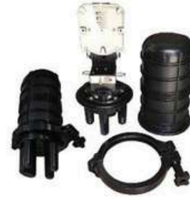
Size: \Phi 140 \times 300.5 \text{mm} ABS Material 48 fibers 3 round & 1 oval port, Heat shrinkable sealing
