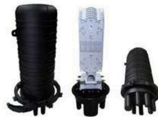
Size: \Phi 168 \times 434.5 \text{mm} PP Material 120 fibers 3 round & 1 oval port, Heat shrinkable sealing
