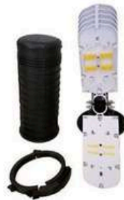
Size: \Phi 230.5 \times 504 \text{mm} PP Material, 144 fibers 6 round & 1 oval port Heat shrinkable sealing
