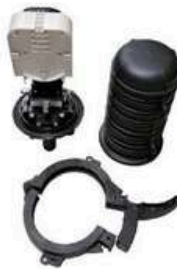
Size: \Phi 146 \times 300.5 \text{mm} PP Material 48 fibers 3 round & 1 oval port, Heat shrinkable sealing
