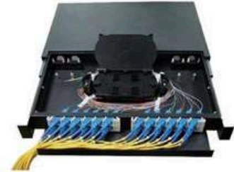
Size:482x317x45.5mm cold roll steel 24 SC simplex 24 fibers
