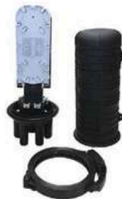
Size: \Phi 146 \times 310.5 \text{mm} PP Material 48 fibers 4 round Port, Mechanical sealing
