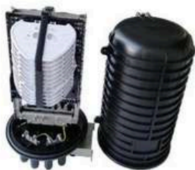
Size: \Phi 304.2 \times 502 \text{mm} PP, 24pcs trays, Max. 288 fibers 1 oval port + 16 round ports Heat shrinkable sealing
